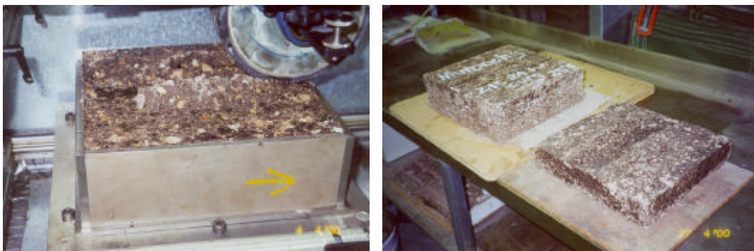
Figure 11 - Wheel tracker test apparatus (left) and foamed bitumen slabs after immediate curing (right) and 24 hours curing (middle).
