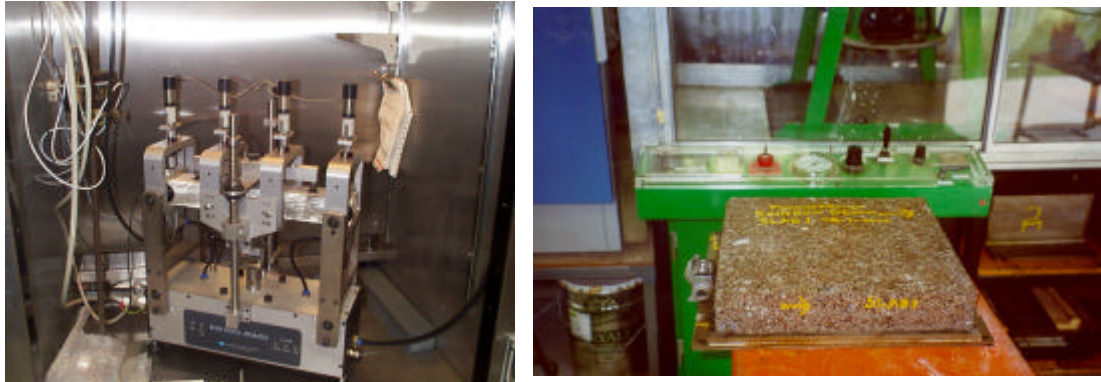
Figure 9 - Fatigue beam testing of a foamed bitumen specimen (left) a foamed bitumen slab (right).
